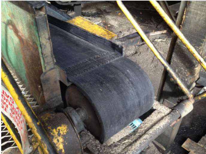
Photo # 4 Conveyor with restricted gate access
