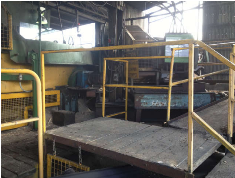
Photo # 5 Steps and platform over chipper conveyor no mid rail
